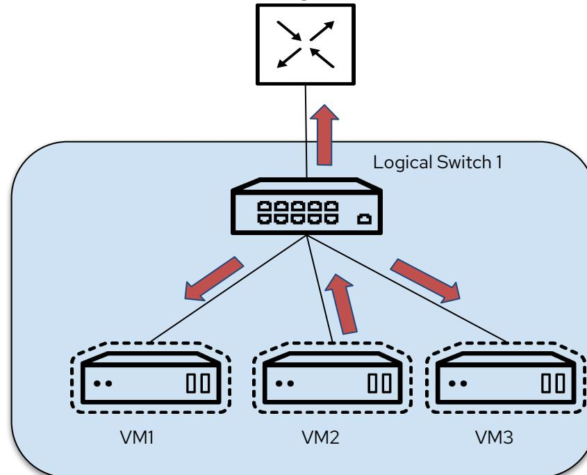
Logical\_Flow: `match=ip4.mcast, action=output(MC_FLOOD)`
